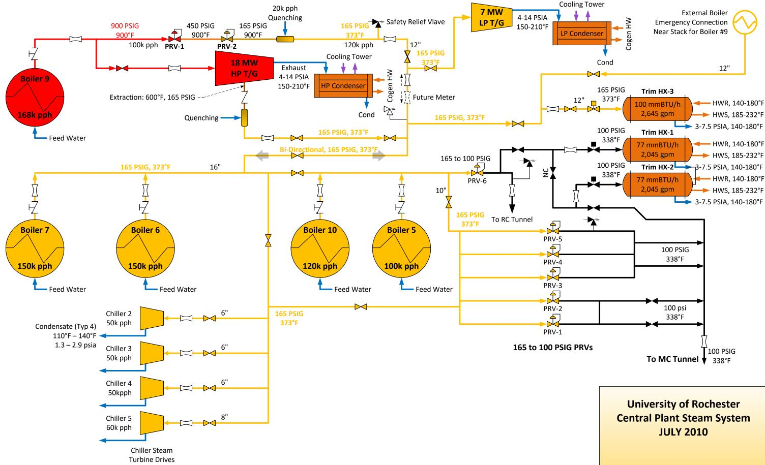
Boilers, 5, 6, 7 and 10 are 165# saturated steam boilers, gas/oil Boiler 9 is 900 psig, 900 F superheated steam boiler, gas/oil
