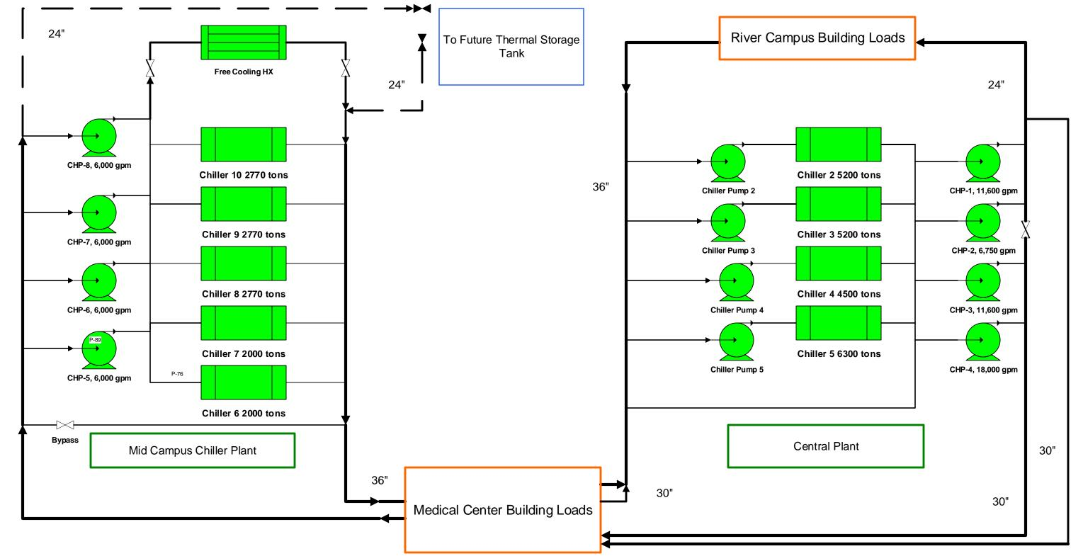
Chillers 2 through 4 are Carrier steam turbine driven chillers, R134 A, 4500 tons, condenser water is from river
