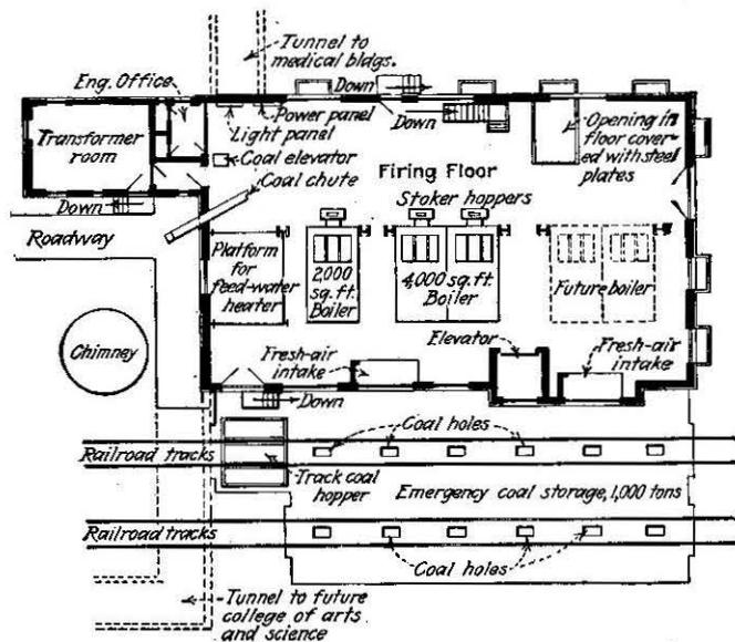
Fig. 5—Floor plan of the boiler house
