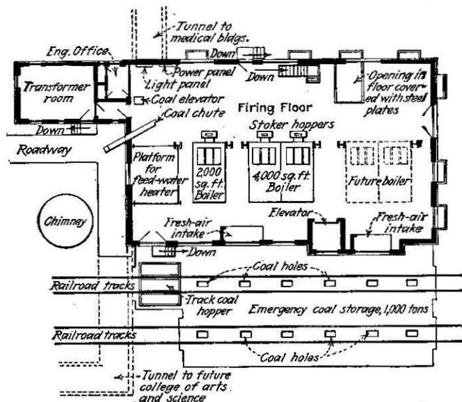
Fig. 5—Floor plan of the boiler house
